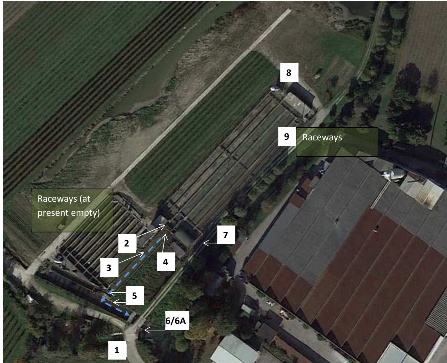
1. Main entrance; 2. Well; 3. Settling tank and water outlet; 4. I° grid up to the settling tank; 5. Jump down to the settling tank; 6/6A. II° grid at the point of water discharge into the Lia stream; 7. Hatchery; 8. Second entrance, silos for oxygen and building for feed storage 9. Raceways;
